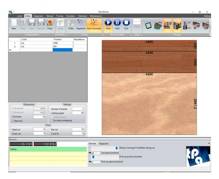
It is only possible to insert rip cuts, the X and Y dimensions of the board are not programmable, and saving the cutting pattern is not allowed.
