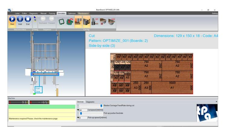
In the 3D view, you will see on the left the three-dimensional model of the machine (its configuration can be provided by the manufacturer), while on the right you will see the 2D graphical preview of the cutting pattern.
