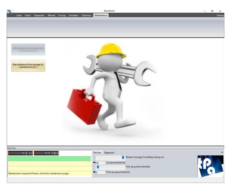
The application allows to define and manage up to 10 programmed maintenance programs; this means that it is possible to set up to 10 machine elements that need to go through regular maintenance. The time for the required maintenance due date can be adjusted to the total operating time of the machine or to the operating time of the main blade. Every maintenance program that is configured in the technological parameters has its corresponding button in the maintenance page.
