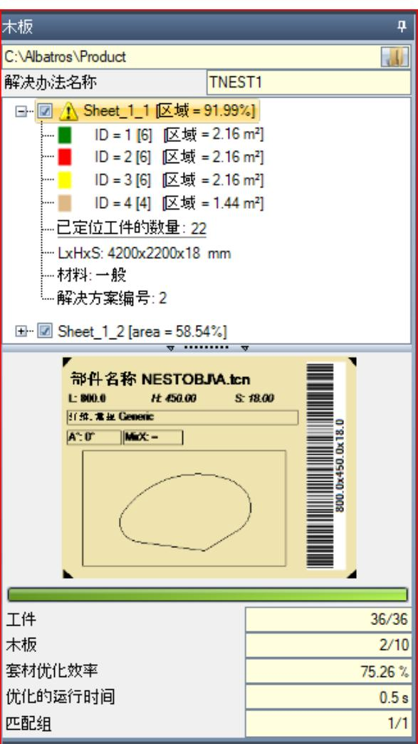
The screenshot shows the 'Nest' panel in TpaCAD. It displays a list of nesting operations for 'Sheet\_1\_1' (area = 91.99%) and 'Sheet\_1\_2' (area = 58.54%). Each entry includes a color-coded icon (green, red, yellow, brown), ID number, and area. Below the list are statistics: '已定位工件的数量: 22', 'LxHxS: 4200x2200x18 mm', '材料: 一般', and '解决方案编号: 2'. A preview window shows a single nesting operation with a barcode and dimensions L: 800.0, H: 450.0, S: 18.0. At the bottom, there's a summary table:
